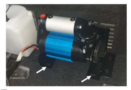
Sit the bracket assembly in desired position on the LH side of the vehicle and mark the centre of the slotted holes with a permanent marker. (compressor temporarily fitted to bracket to ensure correct location).
