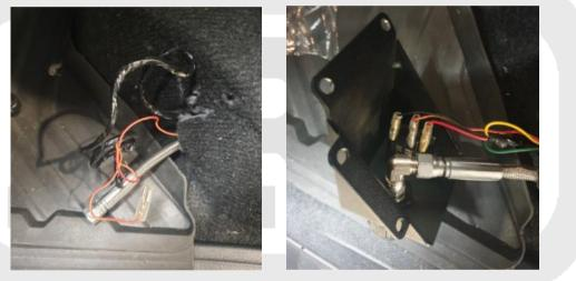
Feed the compressor wiring and air line through the cut carpet and connect to the switch and air coupling. The air line will need a 0740104 90deg elbow.
