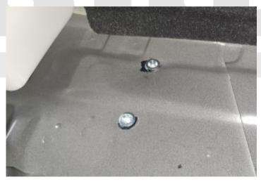
Ensure nutserts have not pinched the carpet Vacuum up all debris caused by drilling operations.
