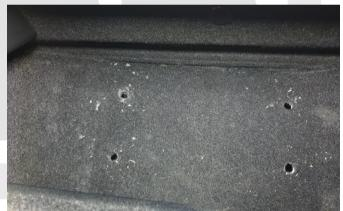
M6 Nutserts need to be fitted to the drilled holes. This can be done with a nutsert gun. Alternatively, the fitting kit comes with a small nutsert fitting device. Assemble the above components as shown. Use a small amount of lubricant between the bolt head and washer.
