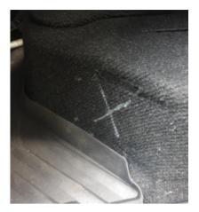
Mark a "X" between the 4x drilled mount holes and carefully cut with a Stanley knife. Behind the carpet is a large hole, where the wiring and air line can be fed from the compressor under the carpet, inside the seat base and then out through the hole as shown.
