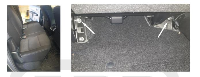
Lift up the rear seat and undo the 5x bolts holding the seat in using a 12mm socket and ratchet.
