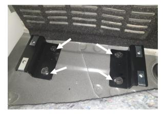
The floor should now look like the above LH image. Remove the mounting feet from the bracket assembly used for marking hole positions. Install the mounting feet as shown in the RH image above, using M6x20 bolts & M6 washers.
