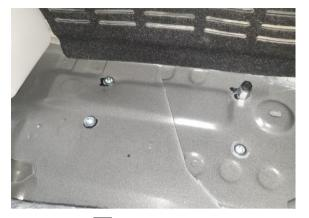
Torque fasteners to 9Nm [7 lbf.ft].
