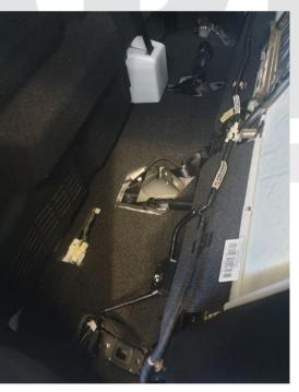
With the help of another person lift the seat assembly and unhook it from the body. Move the seat out of the way and rest it against the front seats.
